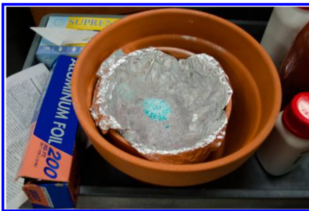
Figure 3. Roman candle ignition mixture added to thermite divot. A second divot is made to accept the \text{H}_2\text{SO}_4 .
