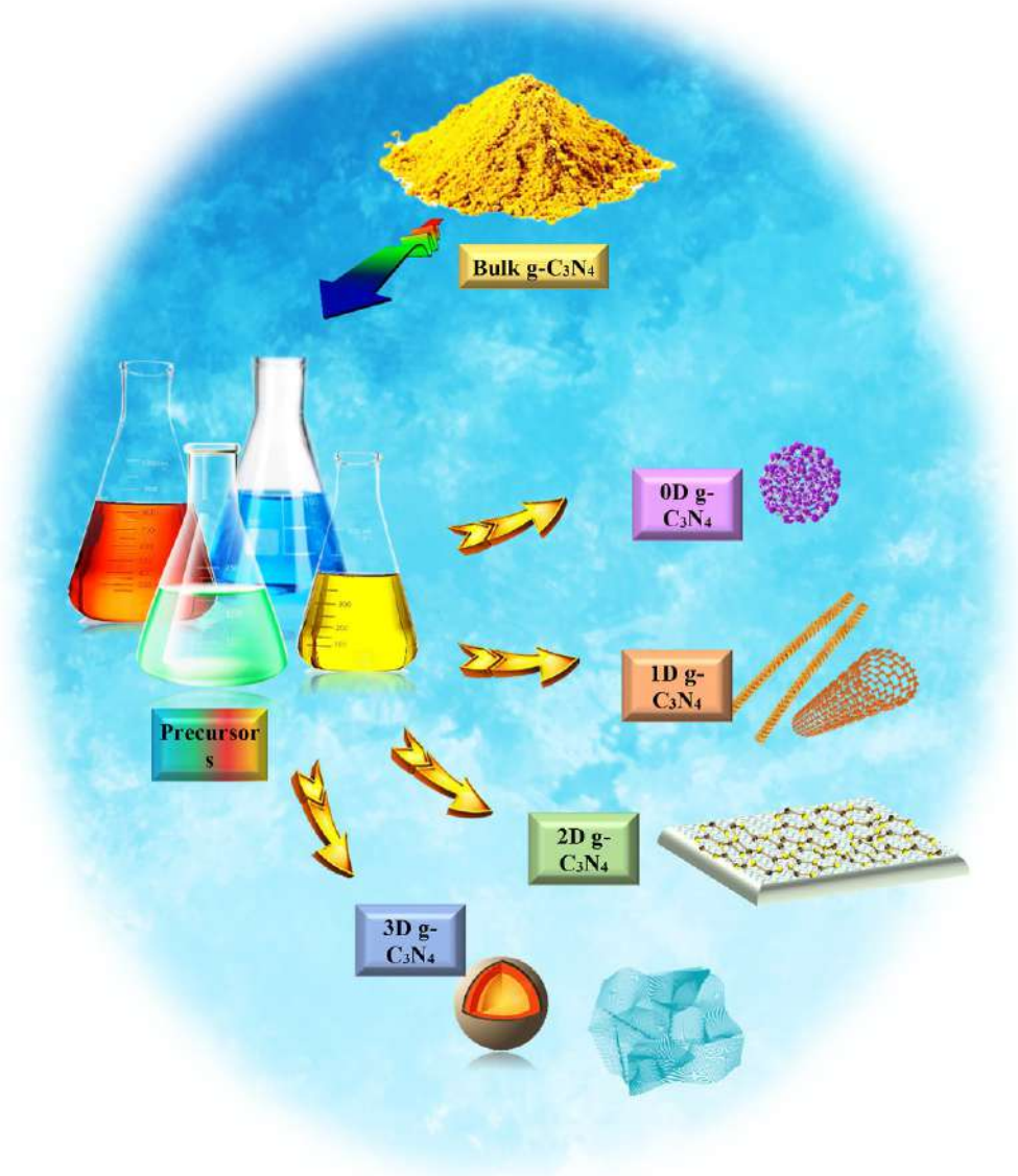
Fig. 8.3 Various dimensionalities of g\text{-C}_3\text{N}_4 which could be produced by utilizing diverse precursors and synthesis methods.
