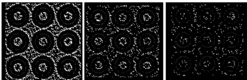
FIGURE 5.2 Hydrogen storage in nanotube bundles. Snapshots from grand canonical Monte Carlo simulations taken under 100 bar pressure at 77 K (left), 175 K (middle), and 293 K (right).
