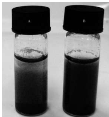
FIGURE 8.4 The dispersibility of SWCNTs–COOH (A) and CD-SWCNTs (B) in water after 10 min.
