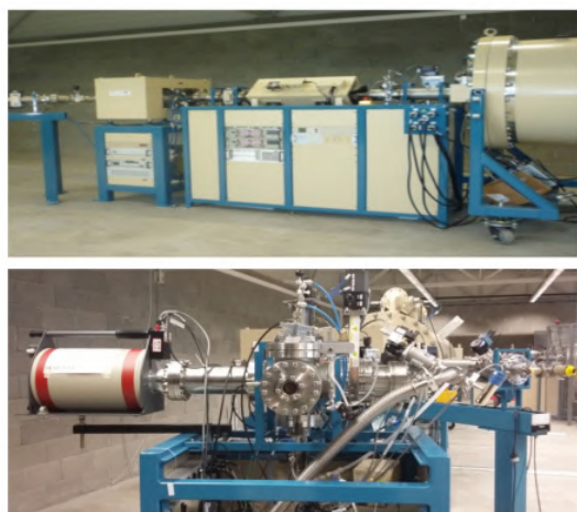
Figure 19: Tandem accelerator laboratory (from the top: Alphasource and SNICS ion sources, injection line, Pelletron, analyzing line with switching magnet, end of the line PIXE/PIGE chamber).
