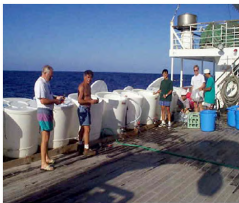
Figure 4: Large volume plastic containers (400 L) on the shipboard for scavenging of ^{90}\text{Sr} , ^{137}\text{Cs} , Pu isotopes and ^{241}\text{Am} from seawater samples (IAEA' 1997 cruise [22]).
