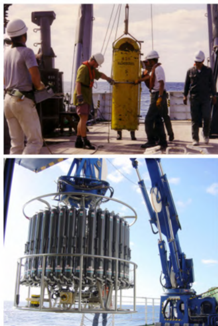
Figure 3: Large-volume (200 L) water samplers (top) compared with the Rosette multisampling system (24 bottles with 20 L volumes) (bottom) operating during deep-water sampling in the Pacific Ocean (IAEA'1997 cruise [22]).
