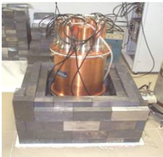
Figure 6: Construction of the anti-Compton gamma-ray spectrometer in the IAEA-EL's Monaco underground laboratory (100% HPGe detector surrounded by NaI(Tl) detectors in a lead shield).
