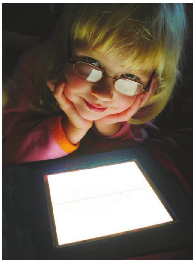
Fig. 28.8. OLED lighting is a very promising new and efficient flat light source based on organic compounds. The white lighting panel in the photograph is 15 × 15 cm, and was developed by chemists in Europe.
