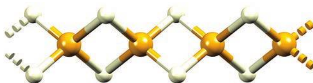
Fig. 10.16. Part of the polymeric chain structure of \text{BeH}_2 ; \text{Be} atoms are shown in yellow.
