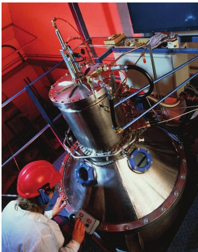
Fig. 6.9. A high-energy gas atomizer used to produce fine metal powders.
