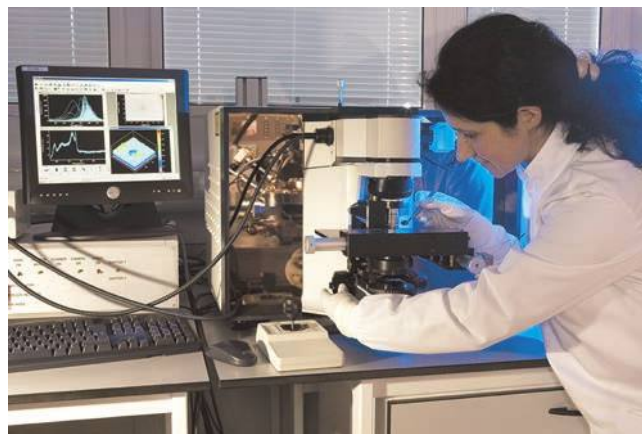
Fig. 4.14. Use of Raman spectroscopy and microscopy. The Raman instrument uses a laser (blue light) to analyse the chemical composition of surfaces of microscopic devices.
