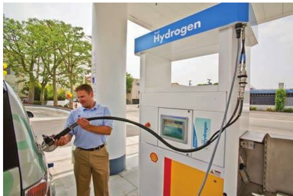
Refuelling a hydrogen fuel cell Chevrolet Equinox in Los Angeles; an electronic plug-in cable controls the refilling process. The vehicle has a range of 150 miles (240 km).
