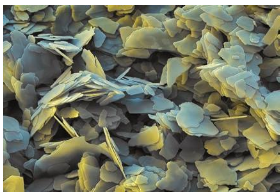
Scanning electron microscopy (SEM) image of TiO 2 flakes. Magnification \times 900 .
