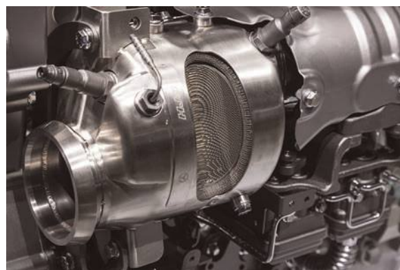
Catalytic converter showing interior design. Small particles ( \approx 1600 pm diameter) of Pd, Pt or Rh are dispersed on a support such as \gamma -alumina which coats a metallic (metalith) or ceramic (monolith) honeycomb-like substrate. The combination of substrate and \gamma -alumina 'washcoat' produces a very large surface area (see Section 25.8).
