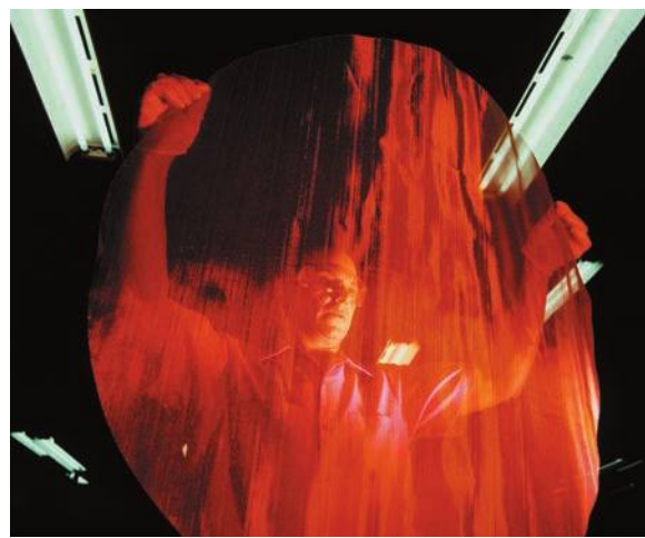
A circular gauze, woven from rhodium/platinum wire for use as a catalyst in the commercial manufacture of HNO 3 by oxidation of NH 3 .
