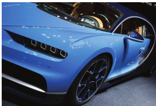
Fig. 28.27. The Bugatti Chiron (unveiled at the 2016 Geneva Motor Show) has a carbon fibre body.
