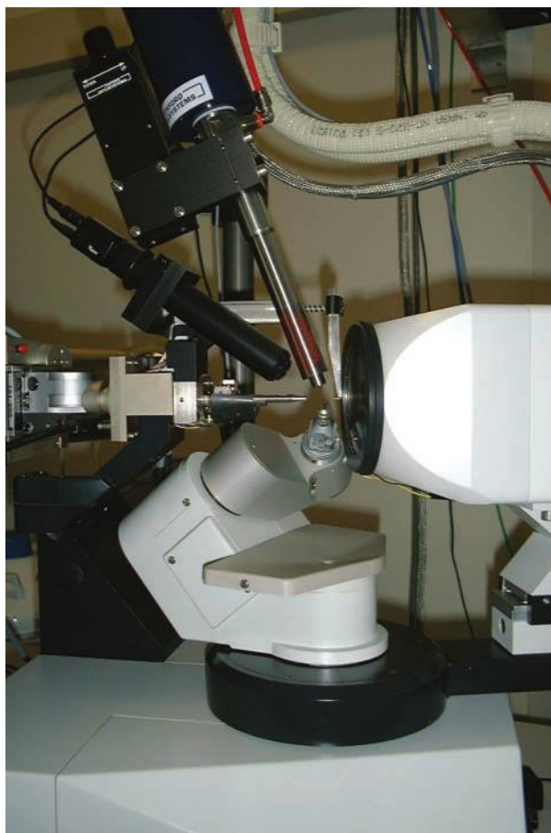
Fig. 4.32. A Kappa-CCD diffractometer equipped with a nitrogen gas, low-temperature cryostat (upper, centre in the photograph). The X-ray source and the detector are on the left- and right-hand sides of the photograph, respectively. The crystal is mounted on the goniometer head (centre). The black 'tube' shown at the upper left is a microscope.
