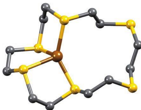
Fig. 21.42. The structure of [\text{Cu}(\mathbf{21.51})]^+ (ligand 21.51 is an \text{S}_6 -macrocyclic) determined by X-ray diffraction for the [\text{BF}_4]^- salt; the \text{Cu}^+ is in a distorted tetrahedral environment [J.R. Hartman et al. (1986) J. Am. Chem. Soc. , vol. 108, p. 1202]. Hydrogen atoms are omitted; colour code: Cu, brown; S, yellow; C, grey.
