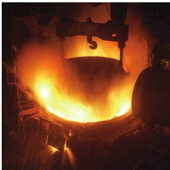
An electric arc furnace receiving a charge of scrap metal.
