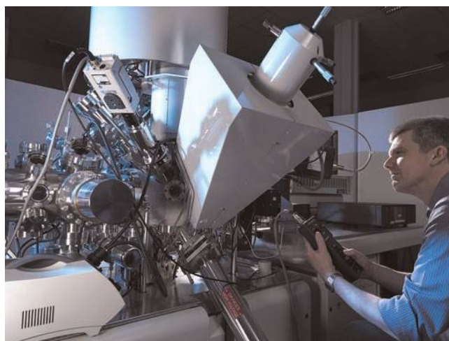
Fig. 4.37. An X-ray photoelectron spectrometer (XPS) being used to analyse the surface of a material.
