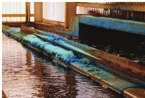
Bioleaching of copper from copper sulfide ores at the Skouriotissa copper mine in Cyprus.
