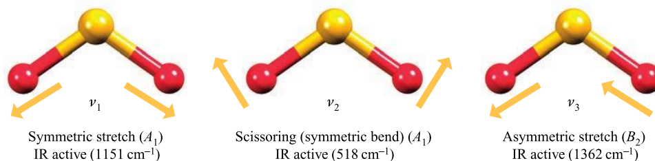
Fig. 3.12. The vibrational modes of \text{SO}_2 ( C_{2v} ). In each mode, the S atom is also displaced from the position shown.
