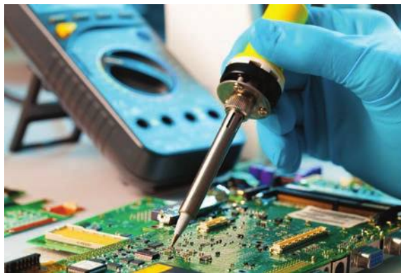
Soldering of chips onto an electronic circuit board.
