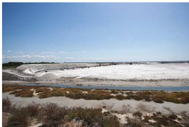
Fig. 11.1. Salt pans and crude NaCl at Salin-de-Giraud in the Camargue, France. Evaporation of water uses solar energy.
