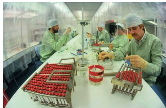
Clean-room assembly of technetium-99m generators. [\text{MoO}_4]^{2-} is adsorbed on alumina in a ‘cold kit’ generator, and radioactive decay produces [\text{TcO}_4]^- .
