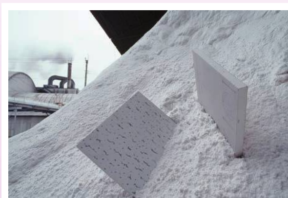
The Yoshino gypsum plant in Japan: recycling gypsum wallboards is an integral part of the manufacturing process which produces new gypsum plasterboards.
