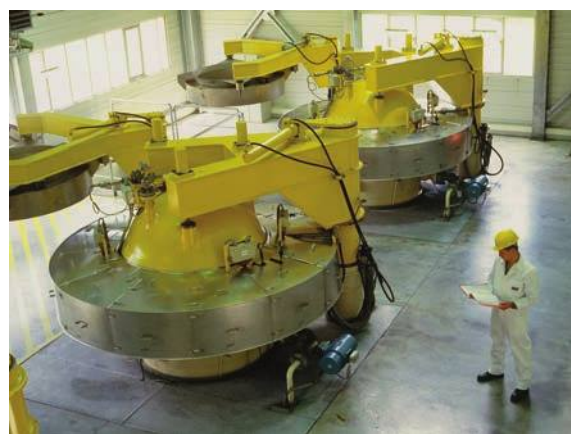
Industrial autoclaves using scCO 2 in a food processing plant.
