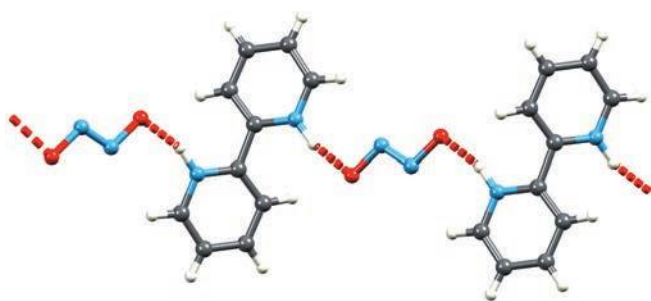
Fig. 15.18. Part of one of the hydrogen-bonded chains in the solid state structure of the 2,2'-bipyridinium salt of [\text{N}_2\text{O}_2]^{2-} . The structure was determined by X-ray diffraction at 173 K [N. Arulsamy et al. (1999) Inorg. Chem. , vol. 38, p. 2716].
