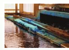
Bioleaching of copper from copper sulfide ores at the Skouriotissa copper mine in Cyprus.
