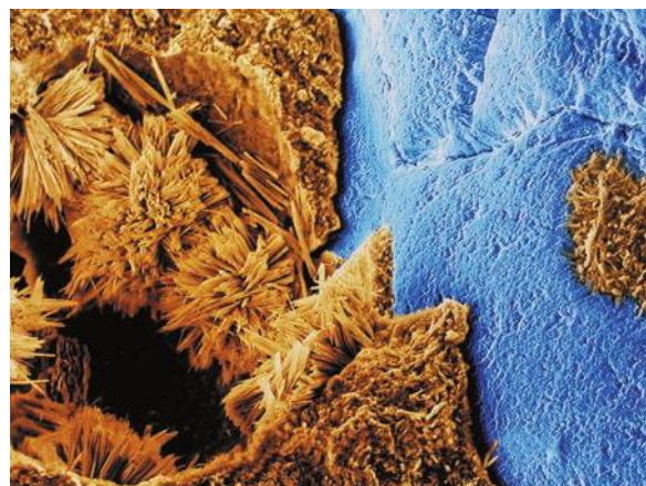
Coloured scanning electron micrograph of gypsum crystals (brown) that have formed in setting concrete (blue).
