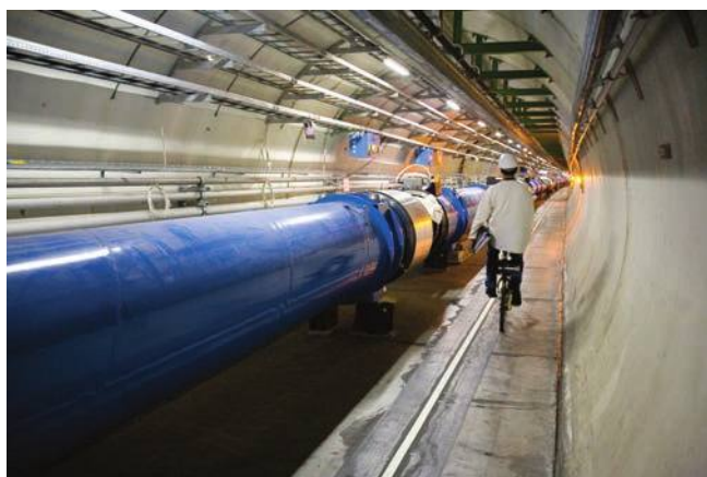
Fig. 28.19. Technician inspecting the Large Hadron Collider which runs in a 27 km tunnel at CERN, near Geneva, Switzerland. The superconducting magnets are housed in the blue pipe-like cryostat.
