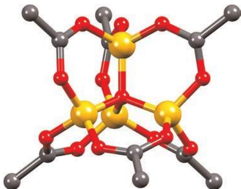
Fig. 12.7. The structure of basic beryllium acetate, [\text{Be}_4(\mu_4\text{-O})(\mu\text{-O}_2\text{CMe})_6] (X-ray diffraction) [A. Tulinsky et al. (1959) Acta Crystallogr. , vol. 12, p. 623]; hydrogen atoms have been omitted. Colour code: Be, yellow; C, grey; O, red.
