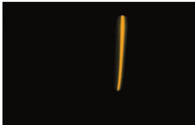
Fig. 1.18. The emission spectrum of sodium. The apparent single line consists of two very close emissions at 589.0 and 589.6 nm.
