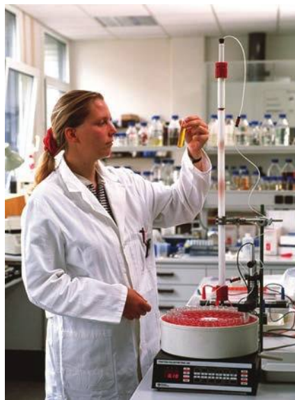
Fig. 4.2. Schematic diagram of an open column chromatography set-up, and an experimental set-up with solvent inlet (top) and fraction collector (bottom).
