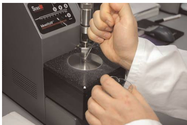
Fig. 4.11. Fourier transform (FT) IR spectrophotometer equipped with a diamond attenuated total reflection (ATR) unit for analysis of solid samples. The instrument shown is being used in a forensic laboratory.
