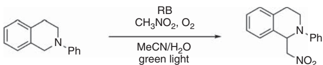
Scheme 3.15 Oxidative amine functionalization by an organic photocatalyst. Source: Pan et al. [50].
