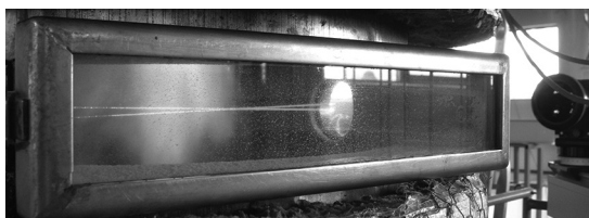
FIGURE 1.10 Laser measurement in the flame (transmitter and crossing of laser beams).
