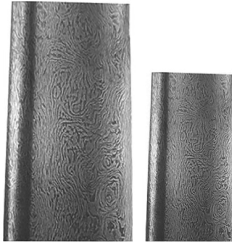
FIGURE 1.2 Damascus steel (Srinivasan and Ranganathan, 2004).
