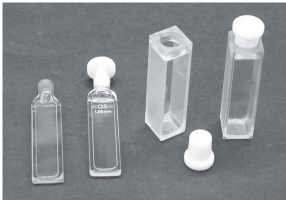
Figure 171. A small set of quartz cuvettes necessary for electronic spectroscopy of the majority of chemical compounds obtained in synthetic laboratories; 1mm and 10mm path-lengths cells with Teflon stoppers.
