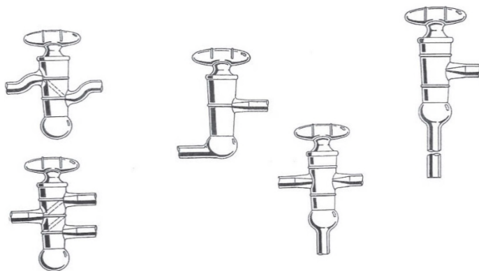
Figure 59. High vacuum stopcocks; 2- and 3-way, with hollow plugs.
