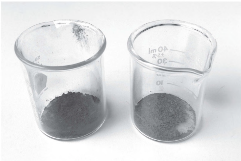
Figure 99. Two batches of dried \text{Cu}_2\text{O} samples obtained from the same reaction: red-colored precipitate (on the left) filtered first, within an hour, followed by golden-colored (on the right) filtered second.
