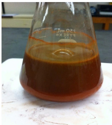
Figure 96. The reaction mixture after addition of hydrazine hydrate, purged with \text{N}_2 and cooled to room temperature.
