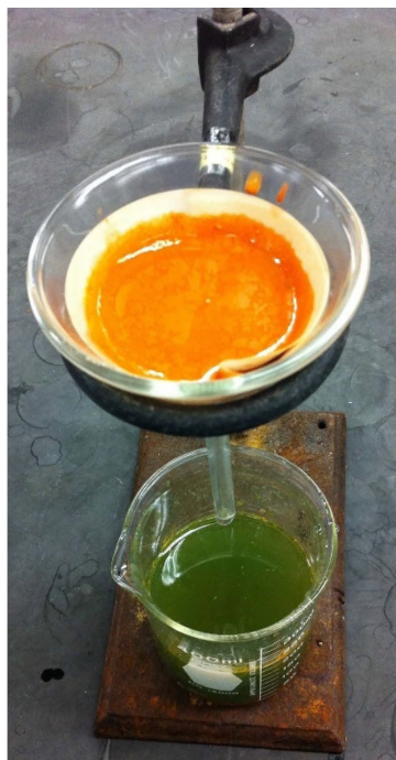
Figure 98. Gravity filtration of the reaction mixture using dense and thick paper filter.
