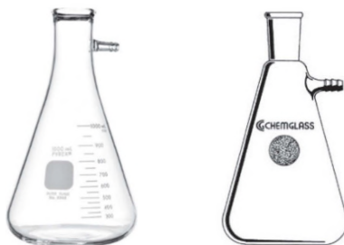
Figure 47. Büchner flasks for filtration. Barbed suction ends (side arms) are designed for tight soft rubber vacuum hose connection.
