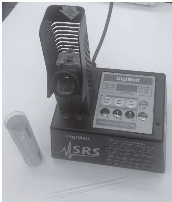
Figure 42. Apparatus for measurement of the melting/decomposition points of chemical compounds. Shown are Pyrex glass capillaries for samples packing.
