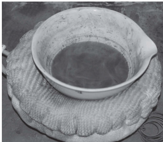
Figure 84. Boiling of \text{MnO}_2 with nitric acid to assure completeness of \text{Mn(II)} nitrate decomposition.
