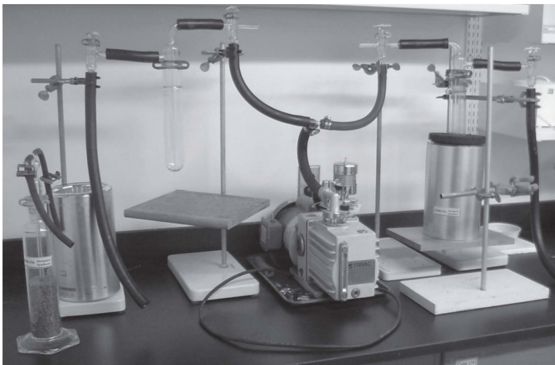
Figure 113. Vacuum station with two outlets for drying of synthesized compounds from residual \text{HCl} and \text{SO}_2 , which can be used simultaneously for conditioning of \text{NiCl}_2 and \text{CoCl}_2 .
