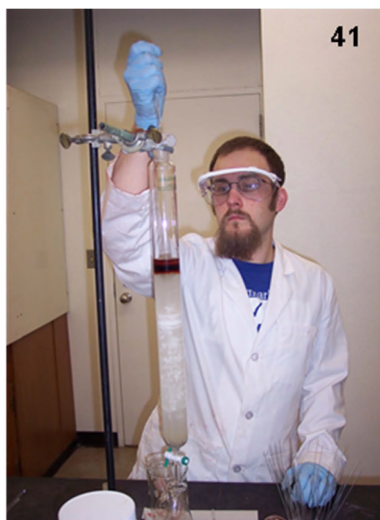
Figure 145. Proper loading of the 'wet' packed column: gloves, a pipette, and careful addition of \text{Co(III)} solution on the wet top of the column for separation.
