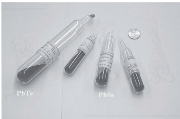
Figure 106. Dry lead(II) halcogenides sealed in glass ampoules under nitrogen for storage.
