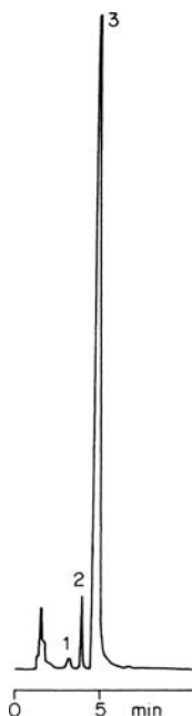
Figure 11.4 Separation of nitrate and bromide in cabbage-lettuce extract on an amino phase. Conditions: sample, 20 \mu l of extract after homogenization, protein precipitation and filtration; column, 25 cm \times 3.2 mm i.d.; stationary phase, LiChrosorb \text{NH}_2 , 5 \mu m; mobile phase, 1 ml \text{min}^{-1} 1% \text{KH}_2\text{PO}_4 in water adjusted to pH 3 with \text{H}_3\text{PO}_4 ; UV detector, 210 nm. Peaks: 1 = nitrile (from nitrate converted during sample treatment); 2 = bromide; 3 = nitrate.
