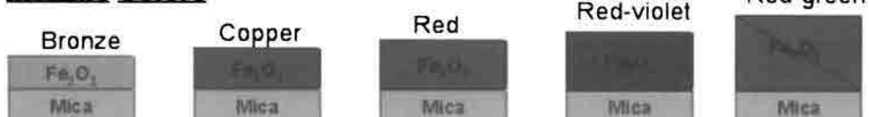
Figure 15.6. Schematic illustration of different metal oxide-mica pigments.
