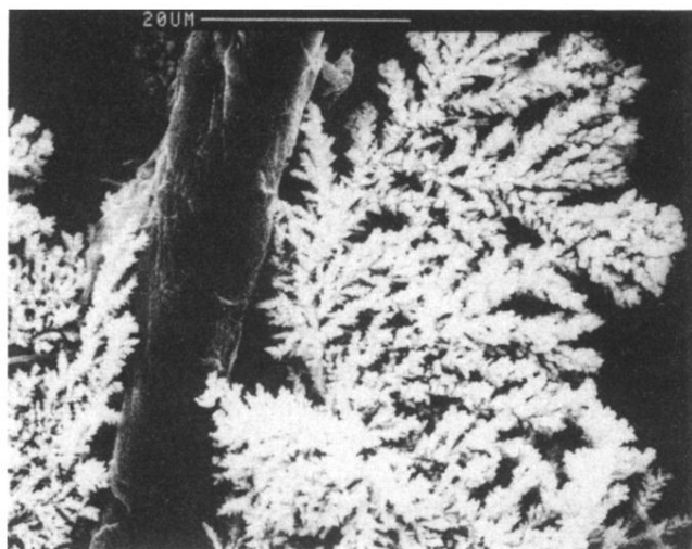
FIG. 8. A growth and fiber from a 3-V growth from 0.75 \text{ mol dm}^{-3} \text{ CuSO}_4 , 1 \text{ mol dm}^{-3} \text{ H}_2\text{SO}_4 . Note that the growth avoids the fiber surface.
