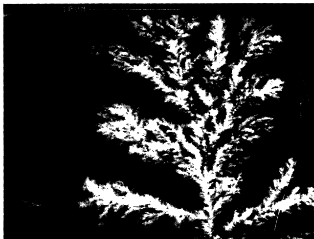
FIG. 12. A growth from 1 V, 0.1 mol dm -3 CuSO 4 , 1 mol dm -3 H 2 SO 4 .
