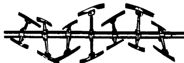
Dry Color agitator construction is used for mixing extremely heavy crystalline or abrasive materials. A series of "T" shaped paddles are spaced 90° apart on the shaft. All except center assembly have one long and one short arm and paddle, effectively circulate material at outer and inner areas of tank; center assembly consists of two long arms to facilitate discharge.
