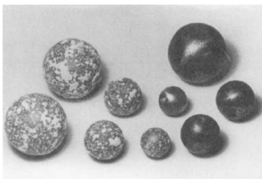
Figure 6.35. Grinding balls before (right) and after brief grinding (left). 2
