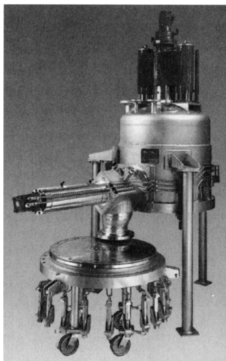
Figure 14.26. Pressure nutsch filter 0.6 m 2 for pharmaceutical pilot plant. Filter is open to show single plate which supports the filter medium (Rosenmund, Inc.).
