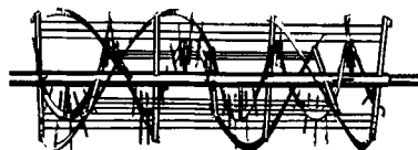
Cut-it-in agitator construction is used for cutting fats, oils and shortenings into flours and powders. Essentially a continuous agitator with cutting bars added to inner ribbon, and cutting wires mounted through ribbon arms. Leather or Tygon wipers are furnished.
