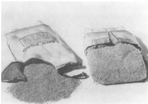
Figure 6.52. Granular fertilizer treated with an anti-caking agent ( left ) and untreated control ( right ) showing severe “bag-set.”
