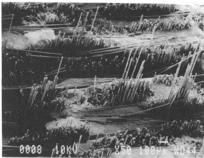
FIGURE 31. Nextel™ 610/ \text{Al}_2\text{O}_3 composite fracture surface following tensile testing at room temperature.
