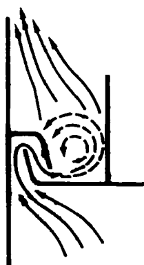
Fig. 264a) Vapour path through collision plates
