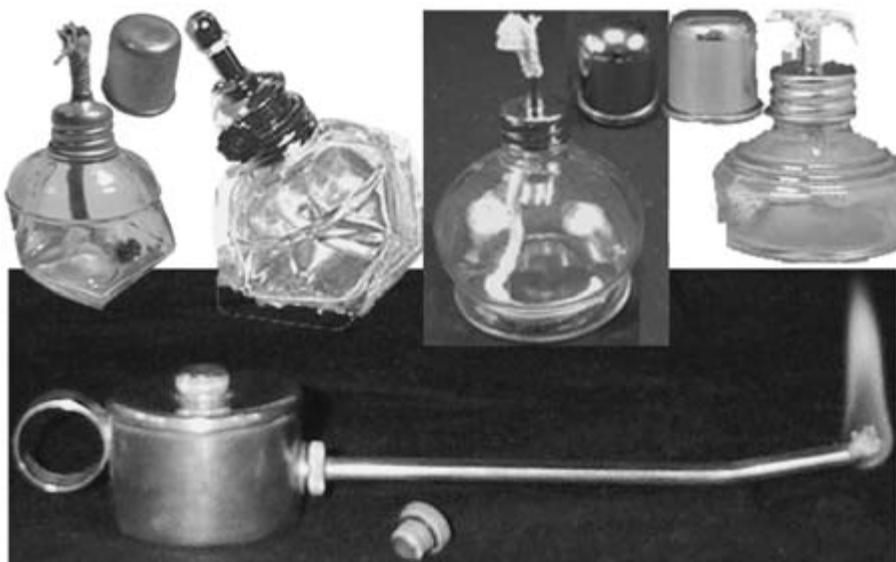
FIG. A1-11. Alcohol lamps or burners.
