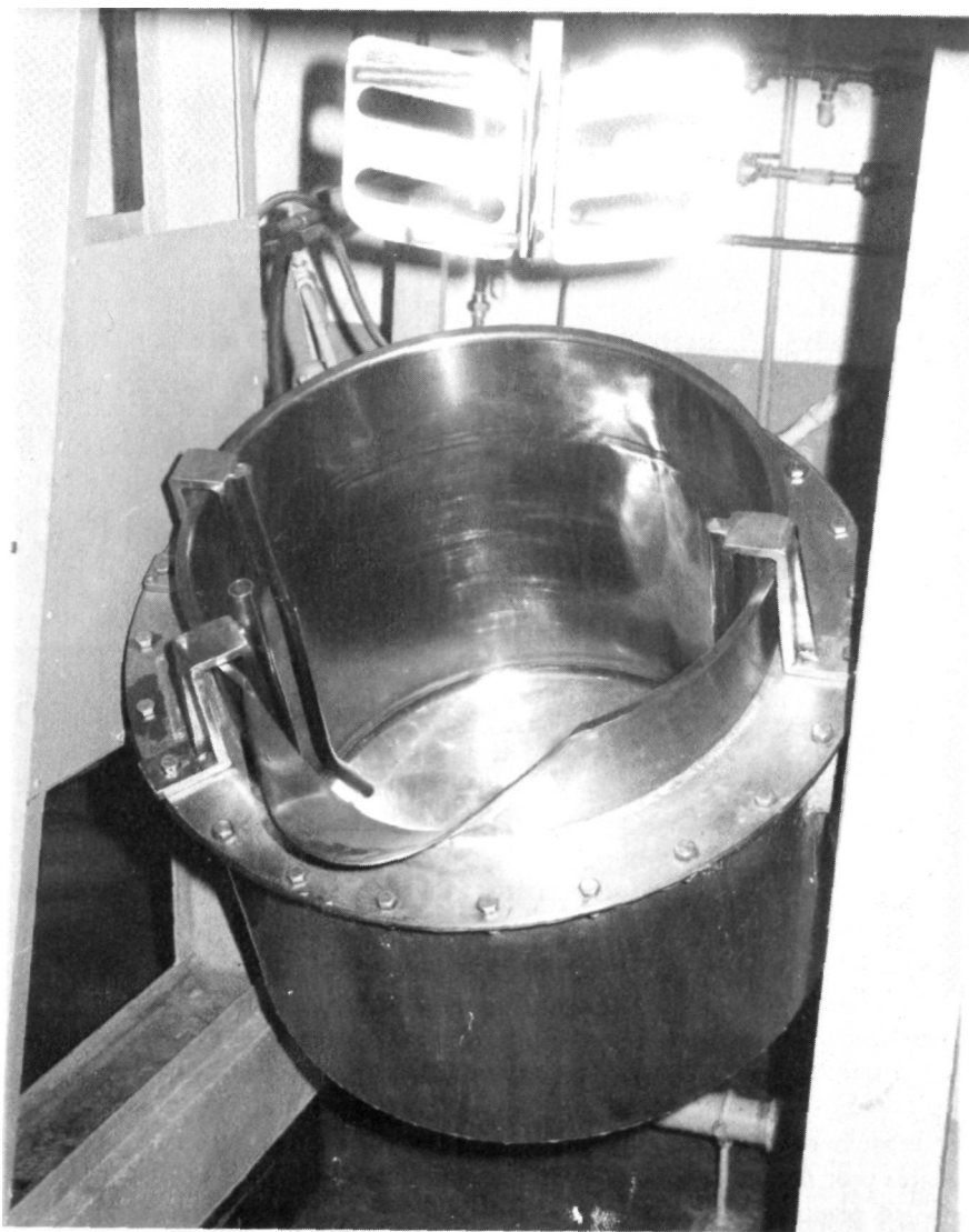
Figure 4. The standard 160-liter vessel used in the U.S. for manufacture of up to 8 kg of lead azide. It is often referred to as "the duPont design" but originated in Germany. The large four-bladed agitator is raised by a wire rope and pulley to permit the tilting of the vessel for discharge of the product.
