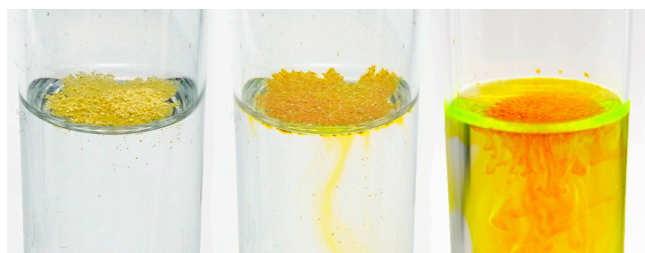
Figure 5. From left to right: fluorescein diacetate immediately after addition to sodium hydroxide solution, after 2 min, and after 5 min.
