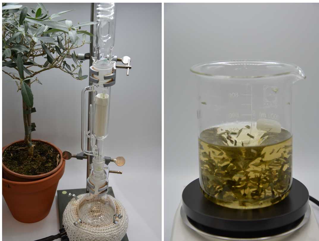
Figure 3. Preparation of the olive solution for the experiments with the Soxhlet extractor and with simple infusion.
